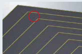
HFC machining without corner movements: rest material in corners
