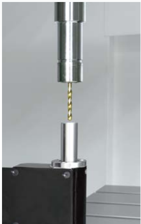
These systems are located behind the ATC cover when not in use. Thanks to this feature, they are protected from chips and coolant during machining.
