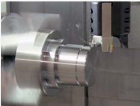
Outer diameter turning (rough) by multiple tool holder
