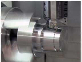
Groove machining by multiple tool holder
