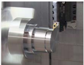
Outer diameter turning (finish) by multiple tool holder
