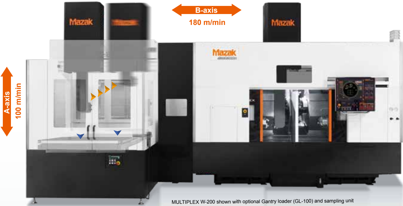
MULTIPLEX W-200 shown with optional Gantry loader (GL-100) and sampling unit
