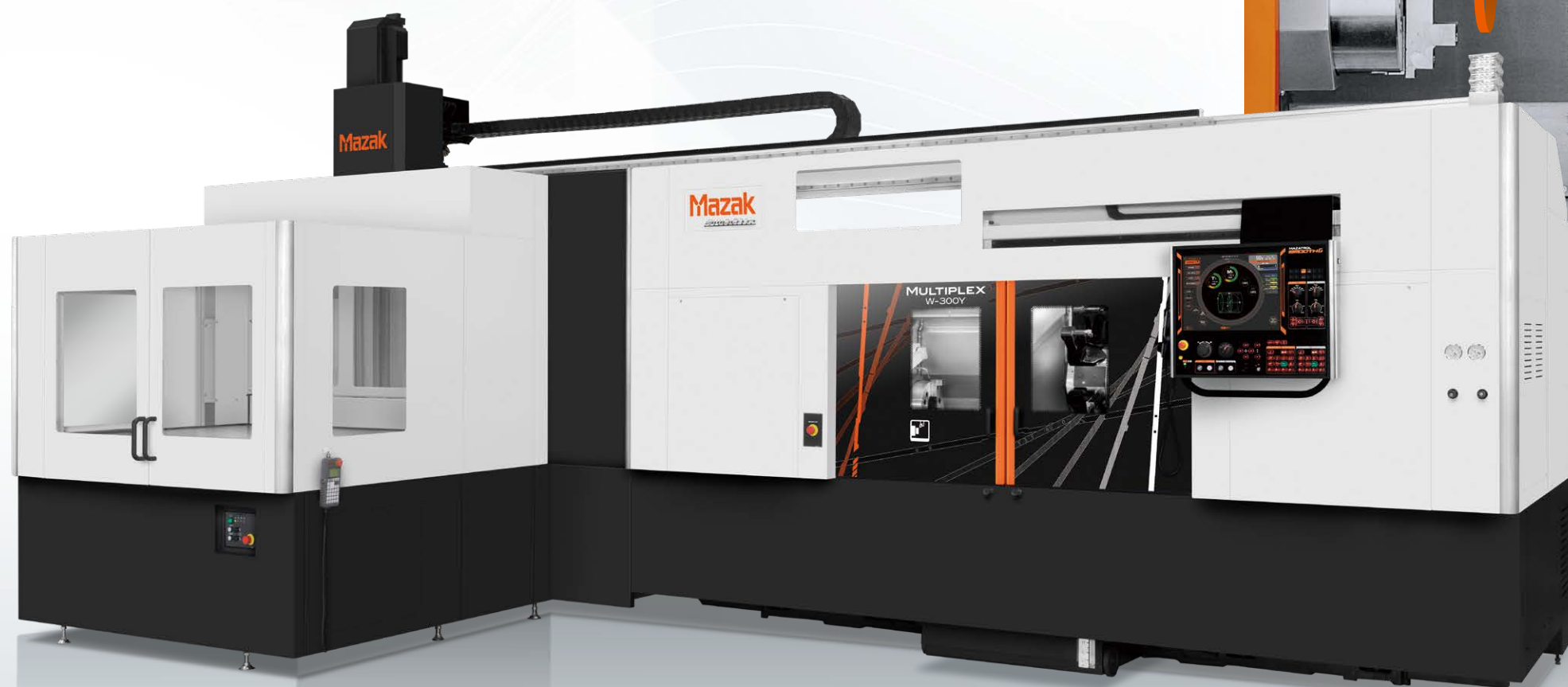
MULTIPLEX W-300Y shown with optionally gantry loader (GL-200) and status light.
