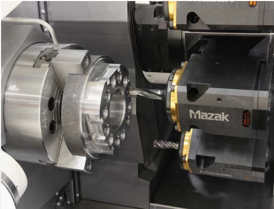
MULTIPLEX W-300, W-300Y 5000 min -1 milling spindle
