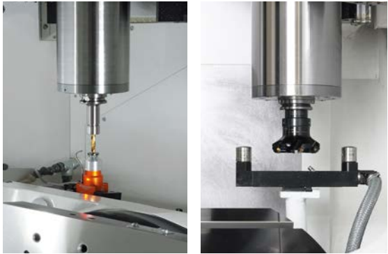
Tool length measurement High-accuracy laser tool measurement system
