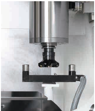
High-accuracy laser tool measurement system
