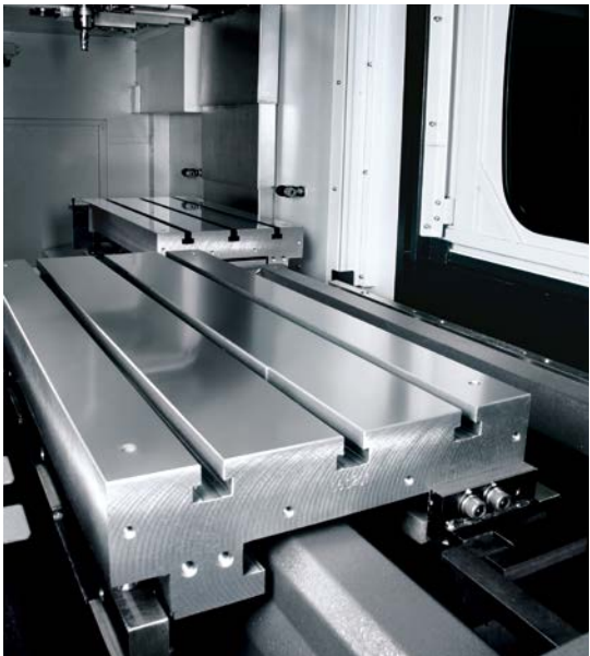
VCN-535C 2-pallet changer (MAZATROL SmoothG)
