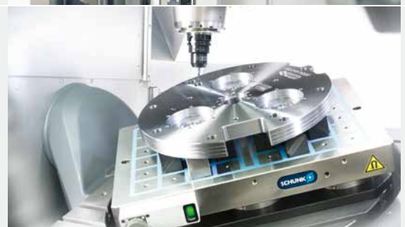
Magnetic clamping technology
